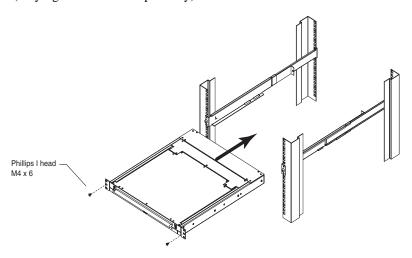
4. Slide the rear attachment sliding brackets along the slide bars until they contact the rear of the switch, then use the screws supplied with this package to attach the bars to the rear of the switch (tighten the screws all the way).
